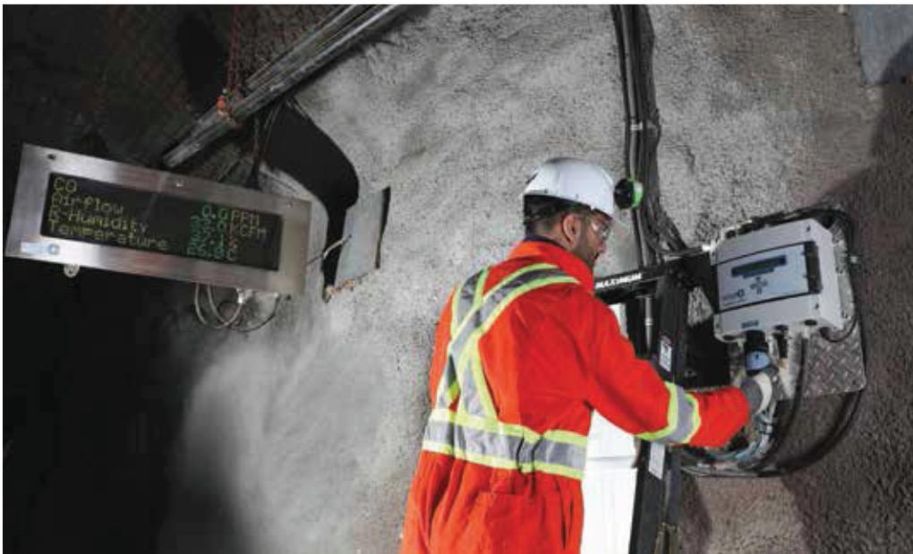
*Maestro designed and developed a digital gas sensor to address the challenges of underground mining.*
