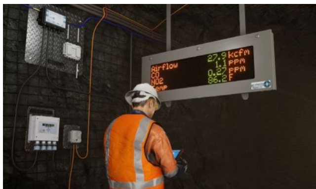
Figure 2. Using the Vigilante AQS airflow rate worker heat stress, humidity, barometric pressure, wet and dry bulb temperature are tracked for health and safety requirements.
