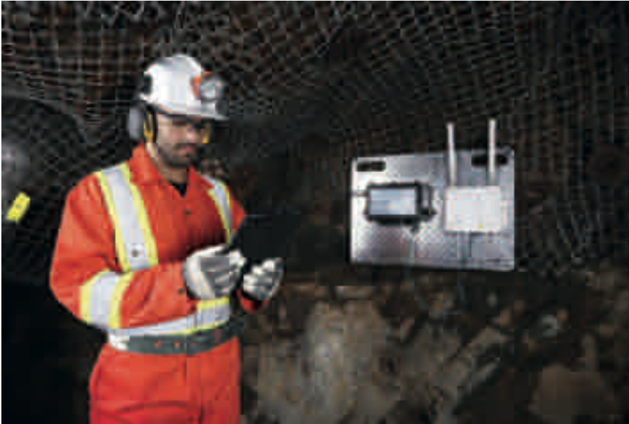
Lundin Gold's new Fruta del Norte underground gold mine in Ecuador integrates Plexus PowerNet™ to enable monitoring of its extensive paste backfill operations
