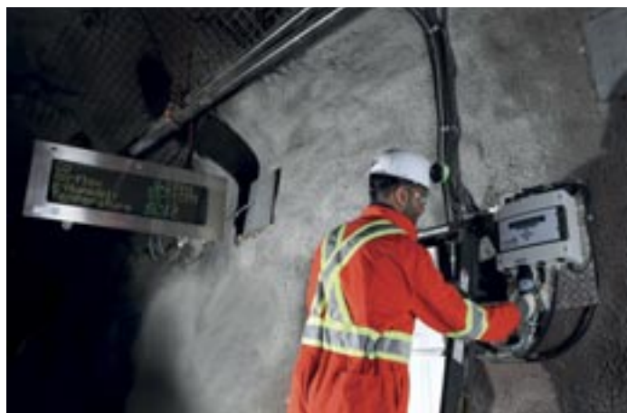
Maestro Digital Mine's Vigilante AQS is a third-generation underground mine air quality monitoring station designed with an improved communication platform
