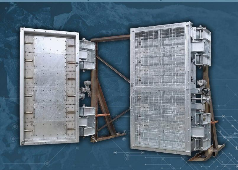
The MaestroFlex™ automated regulators, replacing manual drop board regulators, are designed to exceed underground applications requiring adjustable airflow rates to match changing environmental and mobile equipment demand. The opposing blade design provides optimal flow control over large ranges allowing its use in Ventilation on Demand (VoD) applications.
