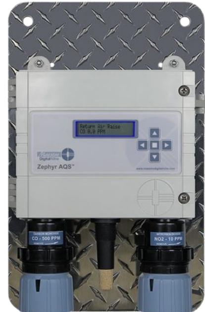
way that the **Zephyr AQS™** communicates over the mine's network using standard network protocols. Maestro fully supports both of the two most popular network communication protocols - Modbus TCP/IP and EtherNet/IP™. Alternately, **the Zephyr AQS™** offers on-board analog outputs (3 x 4-20 mA) and two relay outputs to tie into legacy systems.
