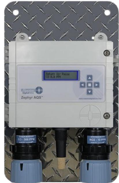
way that the **Zephyr AQS™** communicates over the mine's network using standard network protocols. Maestro fully supports both of the two most popular network communication protocols - Modbus TCP/IP and EtherNet/IP™. Alternately, **the Zephyr AQS™** offers on-board analog outputs (3 x 4-20 mA) and two relay outputs to tie into legacy systems.
